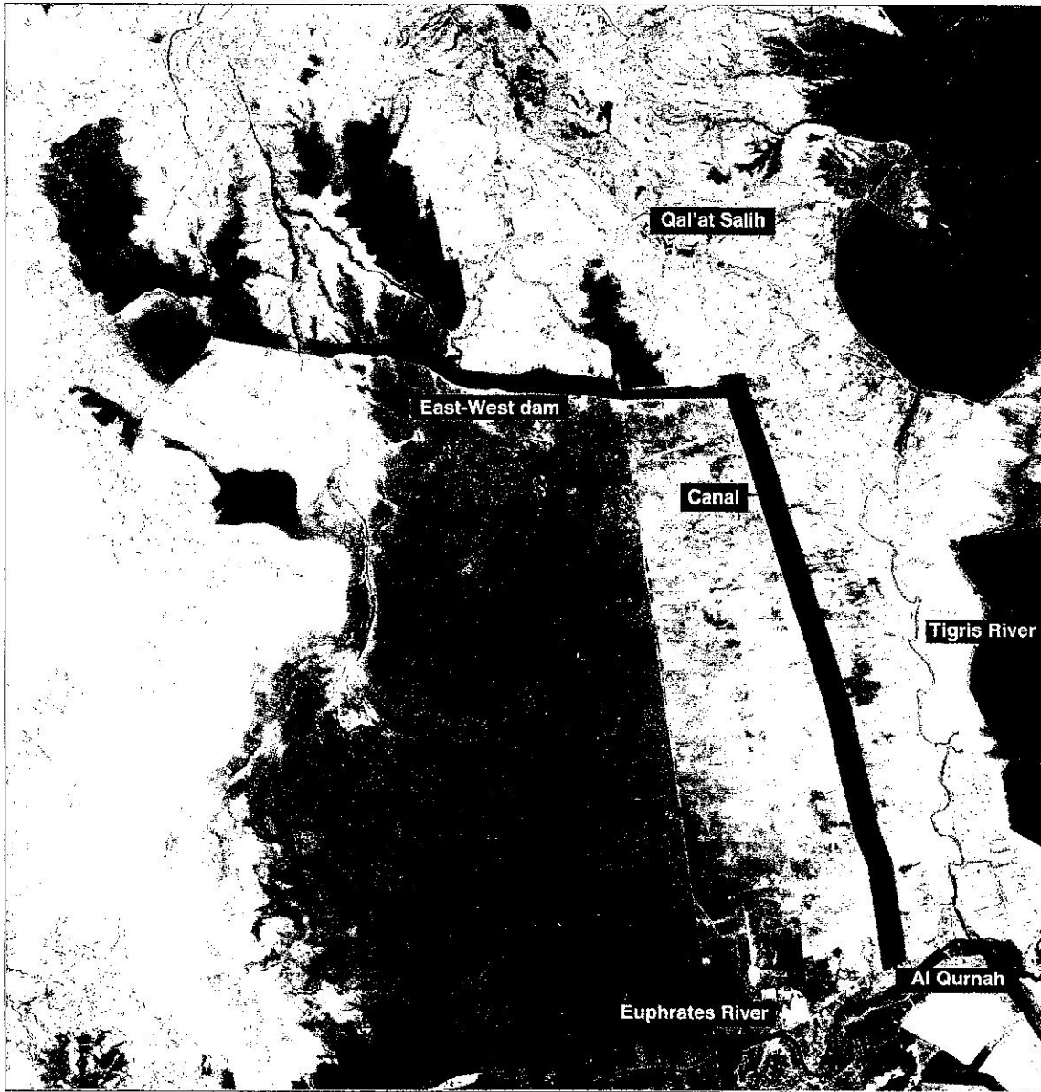
New canal diverting water from the marshes to the Euphrates River.
